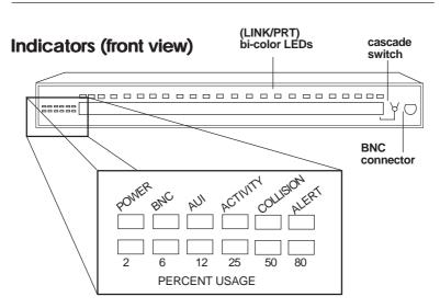
**POWER**: This LED lights whenever power is applied to the BocaNET-24. During normal operation, this light should be ON.
