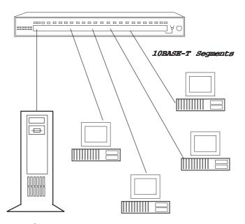
NOTE: File server can plug into any port on the BocaNET-24
