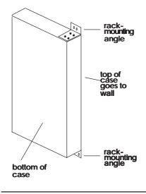
You will need one pair of rack-mounting angles for every BocaNET-24 case you mount to the wall. Attach the 1 1/2" angle portion (4 holes) to two sides of the case using the 4-40 1/4" screws (included). Attach the 7/8" angle portion (2 holes) to the wall. This will require 4 additional screws.
