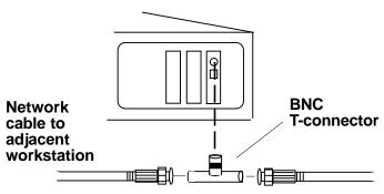
**If YES**, attach a terminator to the open end of the T-connector as shown below:
